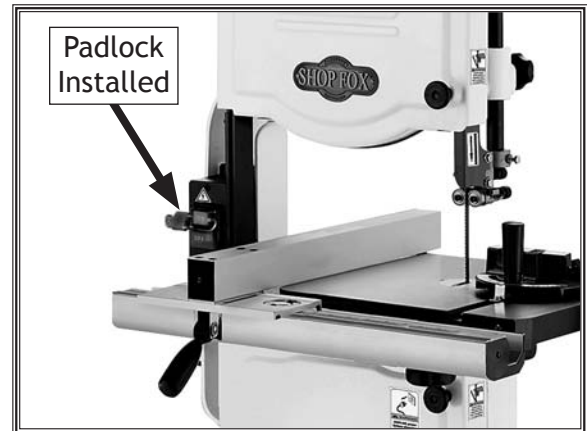
Figure 34. Padlock installed in the switch.
